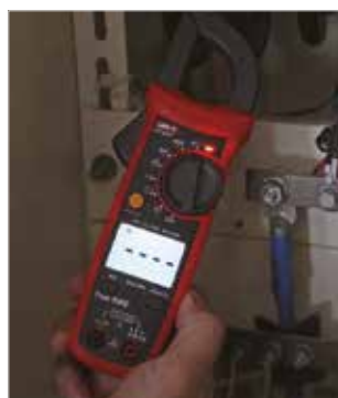
NCV multi-segment display and audio/visual alarm
