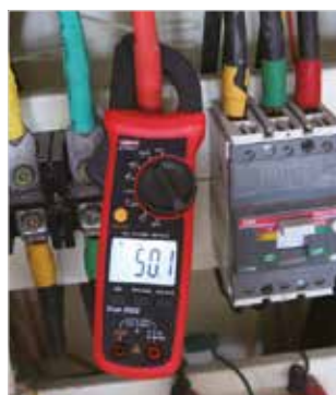
High voltage (600V) frequency measurement
