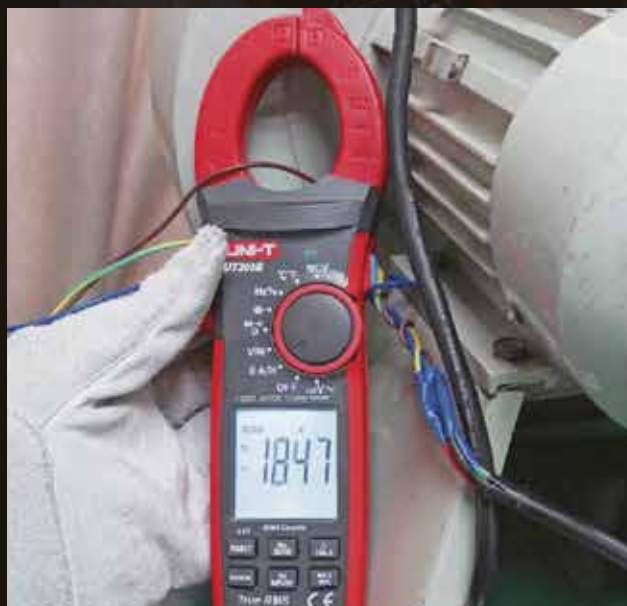
Inrush current capture (UT206B/207B/208B)
