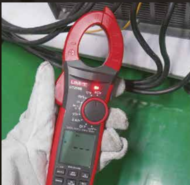
NCV Multi-Segment Display and audio/visual alarm
